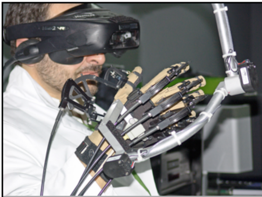
Figure 5 A view of the visual-haptic delivery simulator test-bed, featuring an Immersion CyberForce hand-based haptic device.
